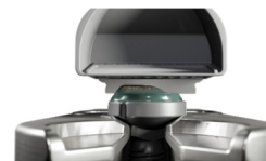
Figure 5. Computer-aided design of the elive™ Edge cutting instrument and its consumables: A) the sample holder, B) the elive™ Edge instrument with the sample holder and blade mounted, and C) the blade holder. Animated images depicting the cutting process: D) the blade sectioning, E) and an example oval LTF.
